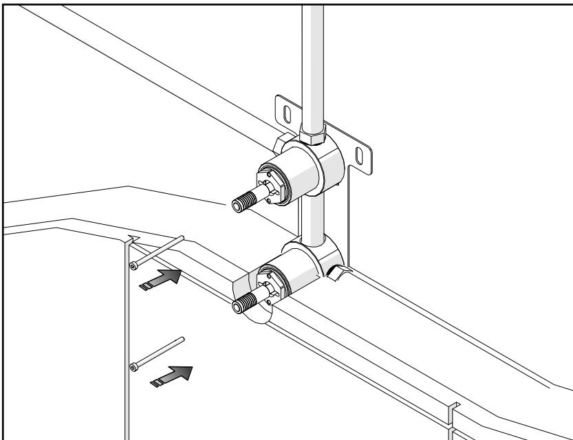
**Fixing of pivot and support for plain washer**
